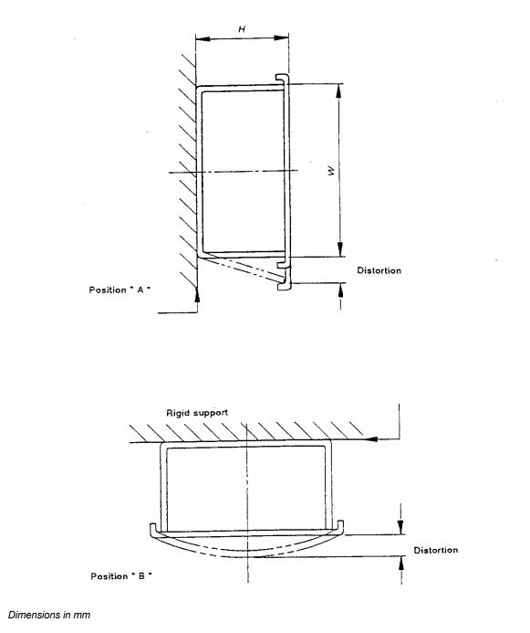
Figure 1 - Cable supporting test apparatus
