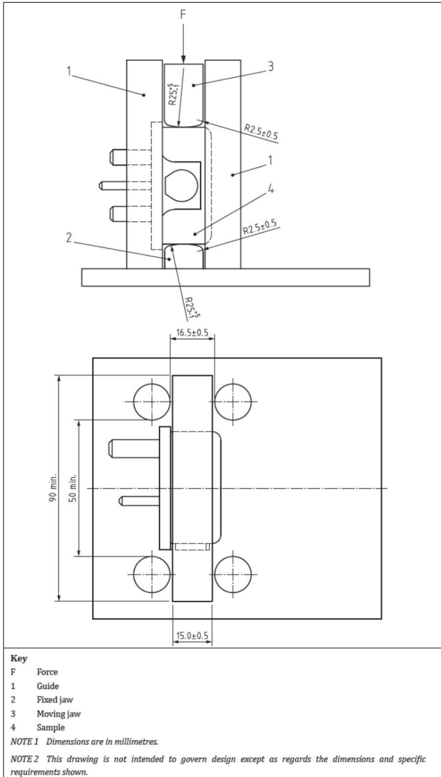
Figure 6 – Apparatus for pressure test (see Clause 25)
